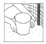
**Step 7.** Pack stones carefully in the bucket to make sure that the water does not run through too fast.
