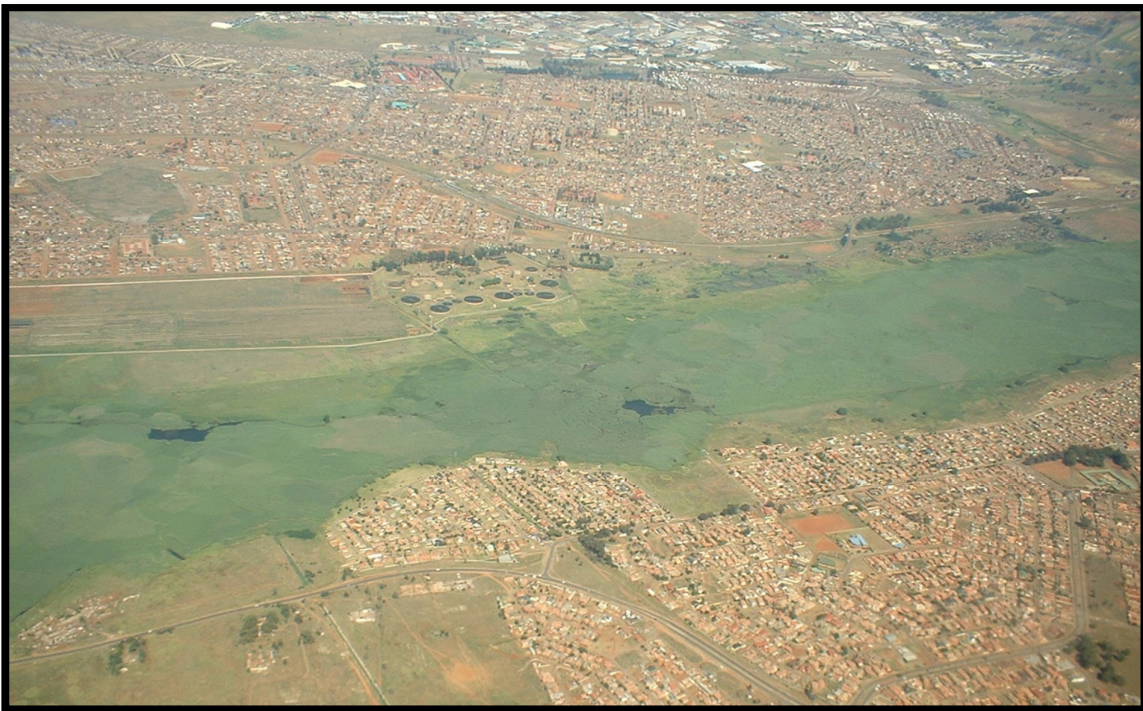
Figure 2: A wetland with extensive built up areas in its upslope catchment, and the considerable discharge of wastewater into the wetland. The wastewater treatment works are visible immediately adjacent to the wetland. The continuous wastewater inputs from this and other treatment works as well as from decanting mines have changed a naturally seasonal system into a continuously flooded system, which has greatly favoured the common reed ( Phragmites australis ).
