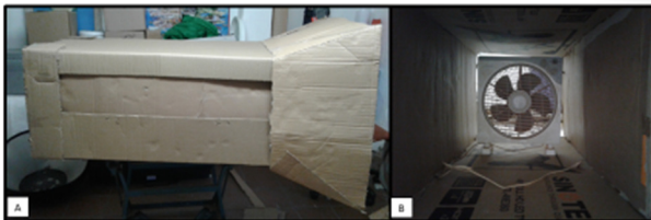
Figure 2.1 A: Side view of a homemade wind tunnel; B: Fan inside the wind tunnel
