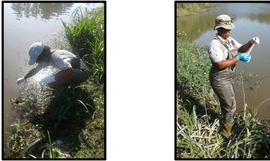
Figure 0.1 Collecting the sample from an area of still water and replacing the swab in the test tube
