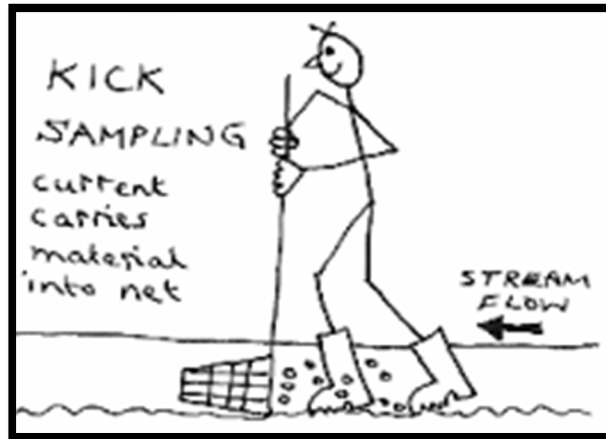
Figure 5: The kick sampling method, the stream current carries material into the net once it has been disturbed by your feet.
