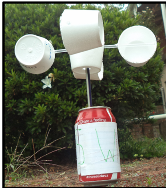
Figure1.1 An example of a home-made cup anemometer, using a cool drink can, a pencil and some Styrofoam cups.
